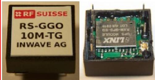
at the same size as the above models the RS-GGO10-TG/T2G also contain a GPS receiver and only need an external GPS antenna. Due to the additional noise and heat generated by the GPS module the typical stability is 1ppb. These modules are mainly intended for applications
