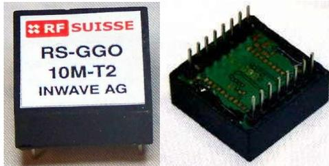
15\*25\*10mm small GPS guided TCXO's with 1PPS input for use with an external GPS receiver. The custom designed circuit enables insensitivity to the quite common errors in 1PPS signals derived from GPS receivers and stability down to 0.5ppb can be achieved. It only requires a steady 1PPS
