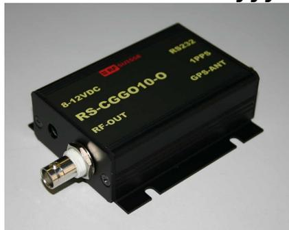
is the same form factor as the above model but is based on the RS-GGO10-O. Except for the significantly improved stability but longer lock time it is feature identical to the above module with the exception of the 1PPS output which continues to toggle with the OCXO accuracy in case GPS lock is lost. Available with 2 different GPS receivers or fibre-optic 1PPS receiver and either BNC or Versatile Link
