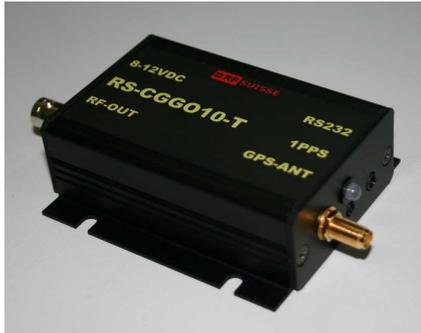
is a reference source based on the RS-GGO10-T with integrated GPS receiver, a full level RS232 to control and read data from the integrated GPS receiver and 50Ω output impedance for the 10MHz output signal. The 1PPS output of the GPS is provided too which is suppressed once GPS reception is lost. Supply voltage is 8-12VDC and can come from an unregulated source. It contains circuitry to
