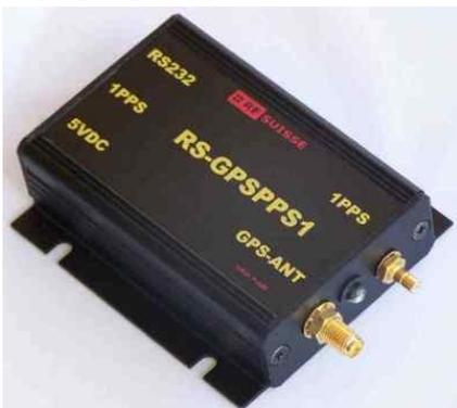
Entry level GPS timing receiver with integrated 1PPS distribution amplifier. This unit is sufficient for most timing applications but only the rising edge of the pulse is GPS controlled. Internal back-up battery and RS232 control of the GPS receiver as well as supply for an active GPS antenna. Four rear and one front 1PPS output. 5VDC supply voltage.
