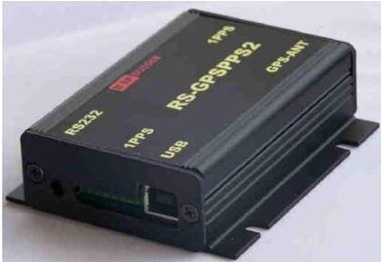
High performance GPS timing receiver with integrated 1PPS distribution. This GPS receiver can be used for all applications where a 1PPS signal is required. The integrated European made GPS receiver can be controlled via USB or RS232. Internal battery backup makes for a fast lock in case of a power failure. The inclusion of supervisory circuits for the
